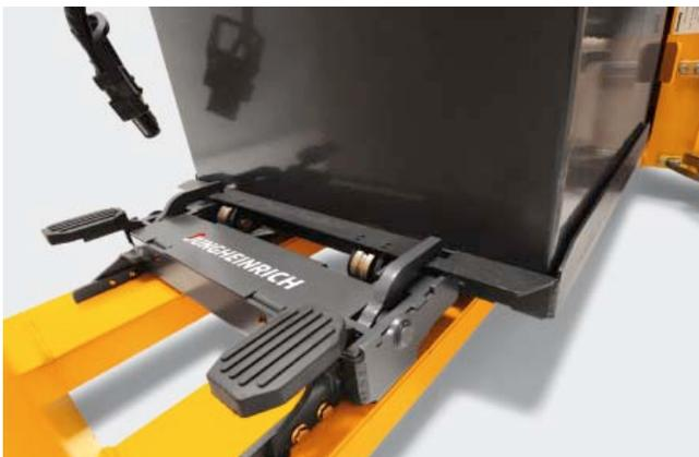
Two side foot notches to open/close the connection with the battery trolley.
