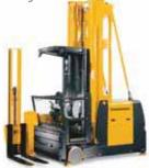
Tri-lateral stacker, **EFX 410–413** max. lift height: 7000 mm max. capacity: 1250 kg
