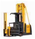
Order picker/tri-lateral stacker, EKX 513–515 max. lift height: 16,500 mm max. capacity: 1500 kg
