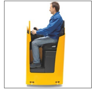
Comfortable seating position with height-adjustable footplate
