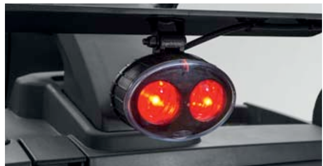
Floor-Spot for safe manoeuvring
