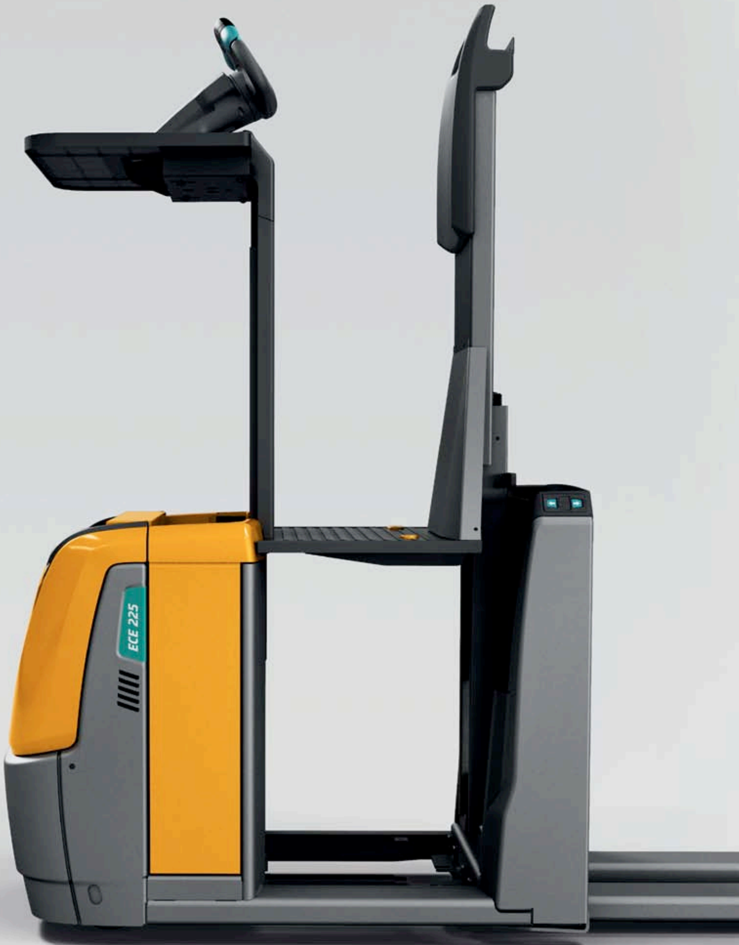
Lifting stand-on platform with control unit (HP-LJ)
