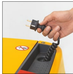
On-board charger also suitable for larger batteries
