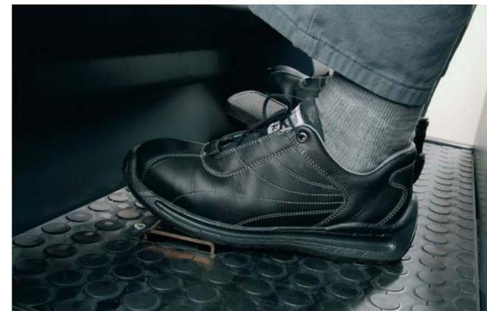
The easily accessible pedal switch for releasing the dead man brake increases the safety for the operator.
